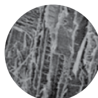
Cell structure – normal kiln dried timber
