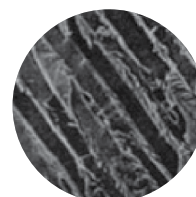
Cell structure – heat tempered timber
